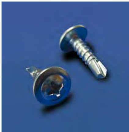
Cixi Zhencheng (profile page 40) Model: SDS02 MOQ: 200,000 pieces Packaging: Carton Delivery: 30 days Price: • Description: Wafer screw; carbon steel; zinc-plated finish; 2mm drilling capacity; 4.2x19mm; 2.09g; DIN
