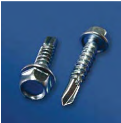
Cixi Zhencheng (profile page 40) Model: SDS01 MOQ: 200,000 pieces Packaging: Carton Delivery: 40 days Price: • Description: Self-drilling/tapping screw; C1018 or C1022 carbon steel; zinc-plated finish; 3.5 to 6.5mm diameter; 1 to 12mm drilling capacity for steel roofing, tapping for wooden materials; ANSI, DIN 7504K, GB
