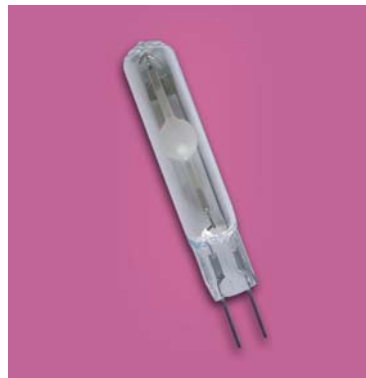
Description: Metal halide bulb; 35W; 90V; 0.53A; 3,300lm/W; 3,000 to 4,200K; 12,000 hours service life; G8.5 base
